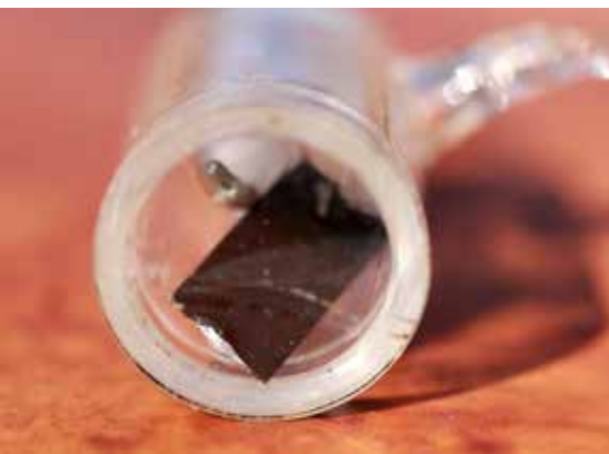
Figure 1. Low's first bolometer. (Photo by George Rieke.)
