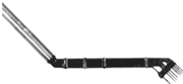
A “rake” with seven electrochemical probes to measure time-varying velocity close to a wall.
