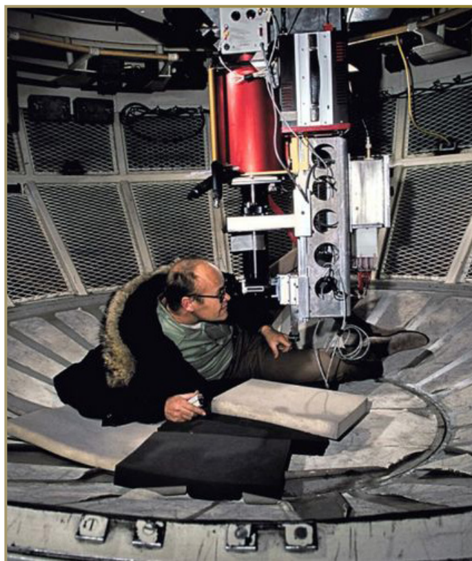
Figure 1 Roger Lynds lying on the floor of the Cassegrain cage at the Kitt Peak Nicholas U. Mayall 4-meter Telescope (1975). The instrument in the cage is a speckle camera, used for high angular resolution work by a clever design that partially compensates for the blurring effect of the atmosphere. Photo courtesy of NOIRLab/NSF/AURA.
